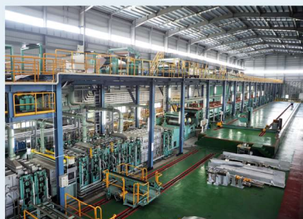
▲ 高產速連續酸洗、清洗、除銹設備 Continuous Pickling, Rinsing, Alkaline Facility
