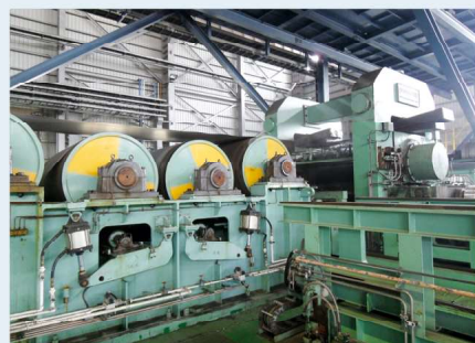
▲ 全自動高強度、高軋下率、調質整平設備 High Reduction rate, Automatic Skin Pass Mill Flatness Facility
