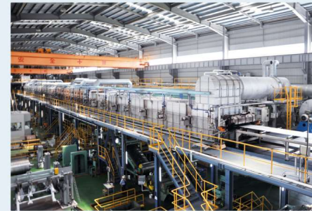
▲ 高效能連續退火爐設備 High efficient continuous annealing furnace
