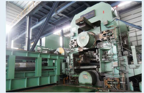
▲ 高張力整平、調質設備 Excellent tension, skin pass mill flatness facility
